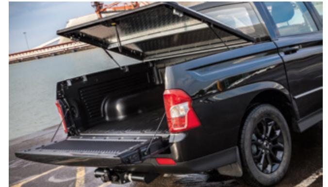
Chequer Plate Top – lockable, heavy-duty alloy chequer plate cover with gas-lift struts and transit tie rails
